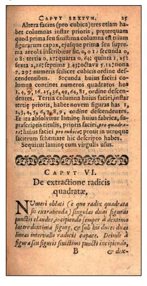
For the square root rod (labelled *pro quadrata*) the left hand column contains (in the same way as the earlier rods) the squares of the integers. The right hand column contains the digits from 1 to 9 while the middle column contains the values that are twice those in the right hand column.
