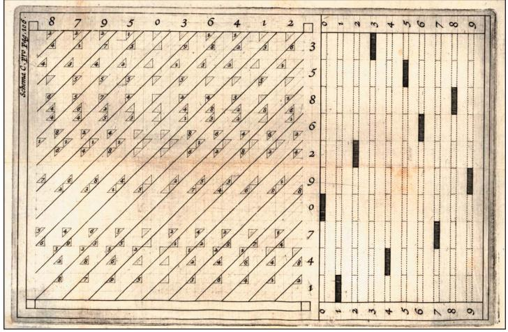
The perforated strips for the multiplier (3,586,290,741) are now placed horizontally on top of the vertical strips for the multiplicand. The right hand portion of this diagram represents the right side of the box with the black areas indicating the storage locations from which the individual strips were drawn.
