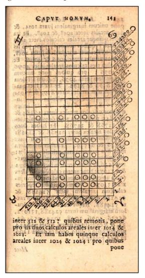
Here Napier provides a second example of multiplying 1,206 times 604 (= 728,424).
