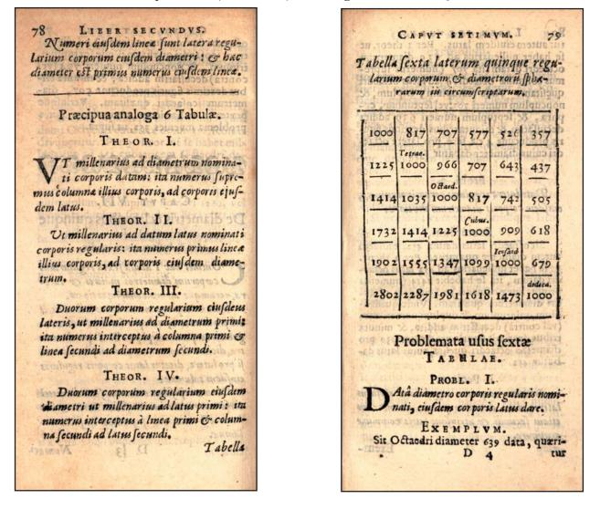
Table six gives the lengths of the sides of regular solids and the diameters of their containing spheres.
