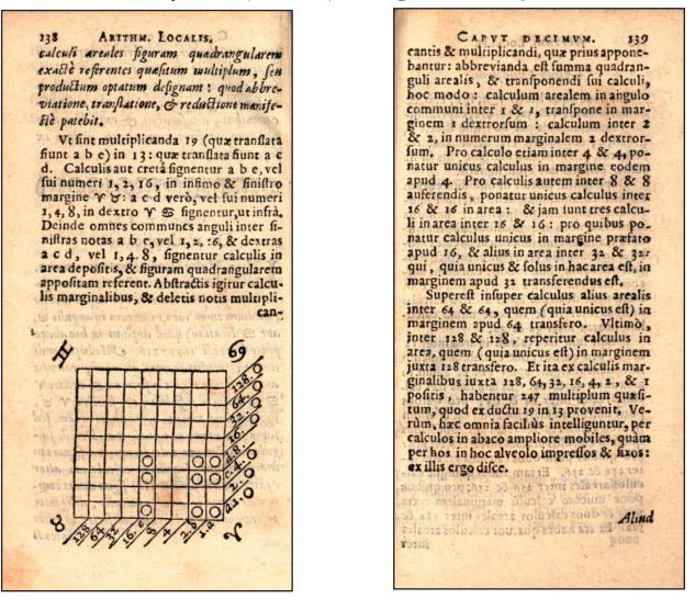
Napier provides the example of 19 times 13. The first number (19) is marked out on the margin of the abacus (in this case he notes this by the letters a,b,e on the  $\gamma$  to  $\Im$  margin) and the second (13) by the letters a,c,d on the  $\gamma$  to  $\Im$  margin. Counters are then placed on the intersecting squares. One must now abbreviate the total shown on the abacus (get it into its canonical form). This is accomplished by moving counters as follows:
