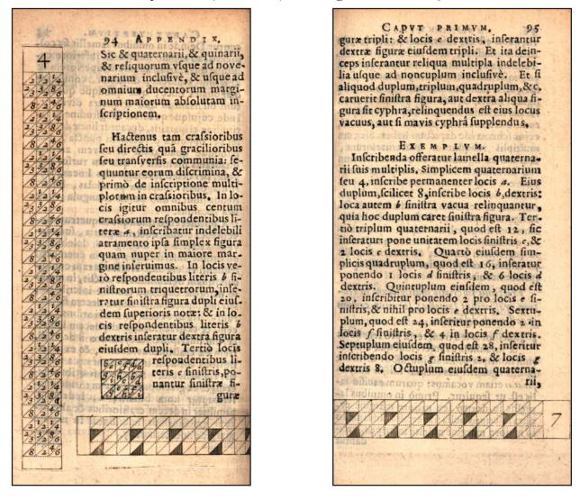
The small square diagram (annotated with the letters a-g in the lower triangle and the letters b-g in the upper triangle) indicates where the various digits are to be placed in the thick strips and the holes in the thin ones.
