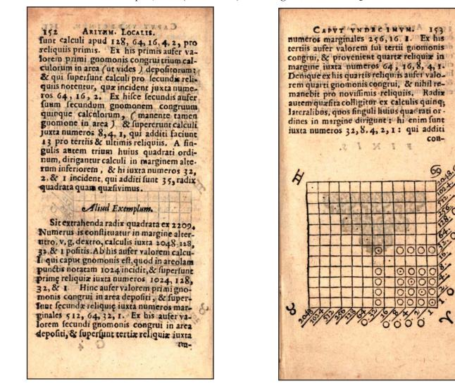
Napier provides a second example for calculating the square root of 2209 (= 47).
