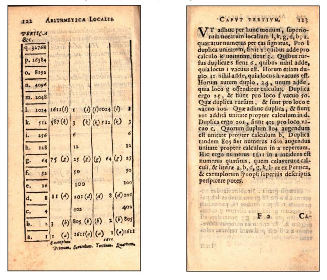
This diagram is simply a representation for the four previous examples and shows the workings of converting and reconverting the number 1611.
