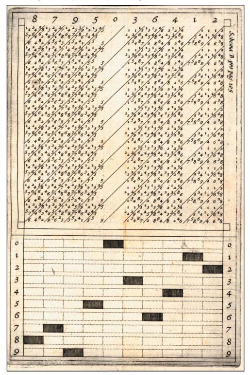
The strips for the multiplicand (8795036412) are placed on top of the box. The lower portion of this diagram is intended to represent the front of the box with the black areas indicating the storage locations from which the individual strips were drawn.
