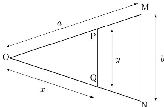
Figure 2: The principle of a sector
