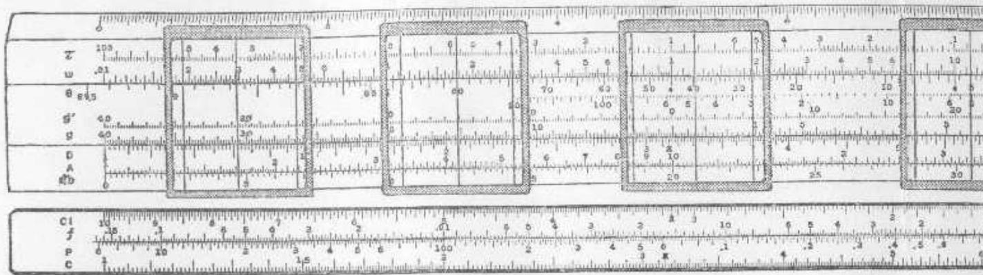
Fig. 1 Slide Rule for Frequency Response Cat. No. 301
