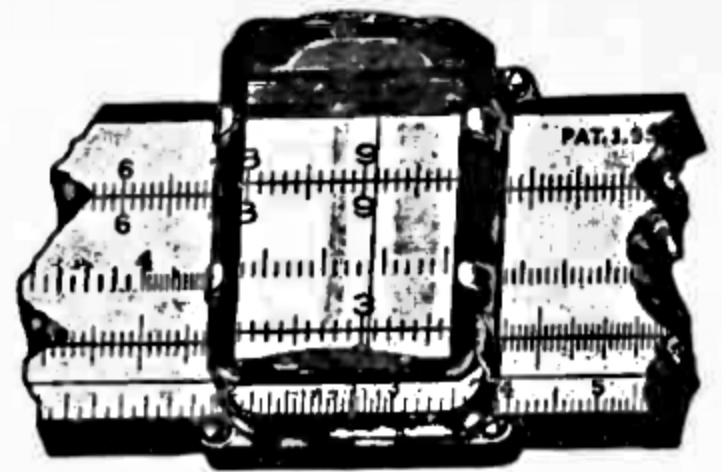
The rule is now set up to multiply 2 by 1.5, to divide 3 by 1.5, or to obtain the square root of 9. A magnifier makes it easier to read accurately.
