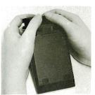
6. Turn calculator over and turn power on to assure proper battery installation. If the display does not light make sure the battery pack is correctly placed in calculator.
