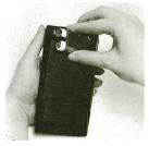
5. Insert battery door and slide door back into place.
