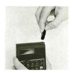
Press down on the battery door where indicated until the door release snaps open. Slide the door open.
