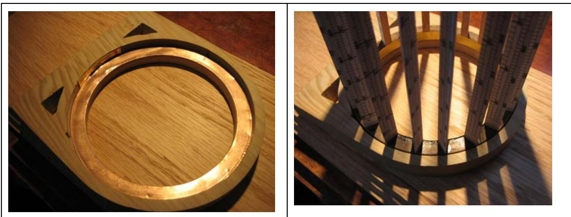
**Figure 9** *And end bracket and the envelope sitting in it.*
