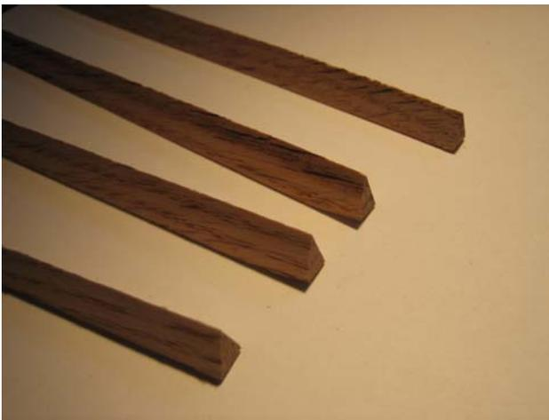
**Figure 5** *Triangular bars  $\frac{3}{8} \times \frac{1}{4} \times \frac{3}{8}$ .*
