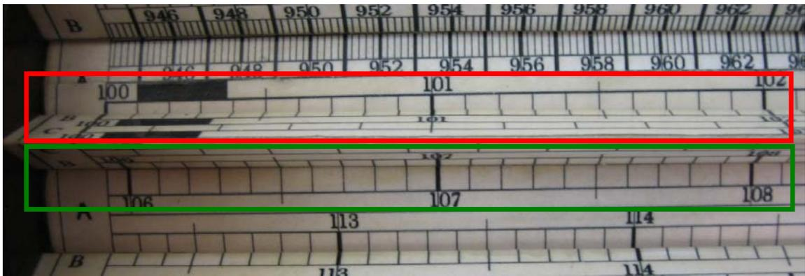
**Figure 1** Close up of the leftmost 3". In the red box, the top of a bar and half the gap above it bear a scale segment that goes from 100 to about 112. In the green box, the bottom half of the same bar and half the gap below it bear a scale segment that goes from about 106 to about 119.
