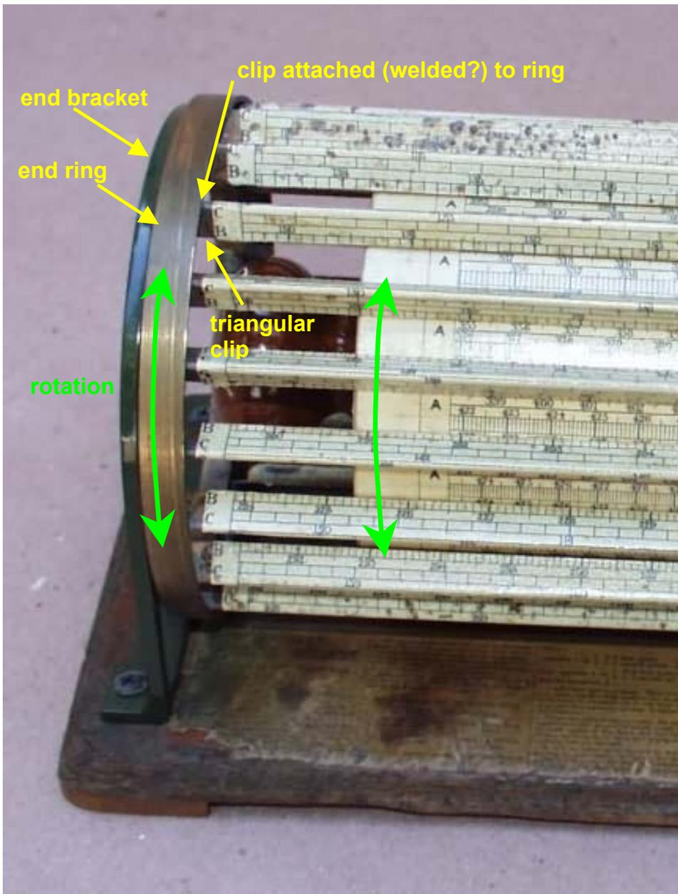
**Figure 2** *The rotating envelope mechanism.*
