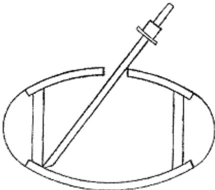
Figure 3. Gauging by the Diagonal Line (from Gauging Instructions, 1932)
