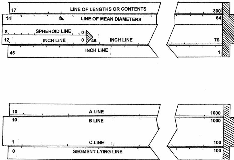
Figure 5. The Head Rod: scheme of lines (face side above, reverse side below)
