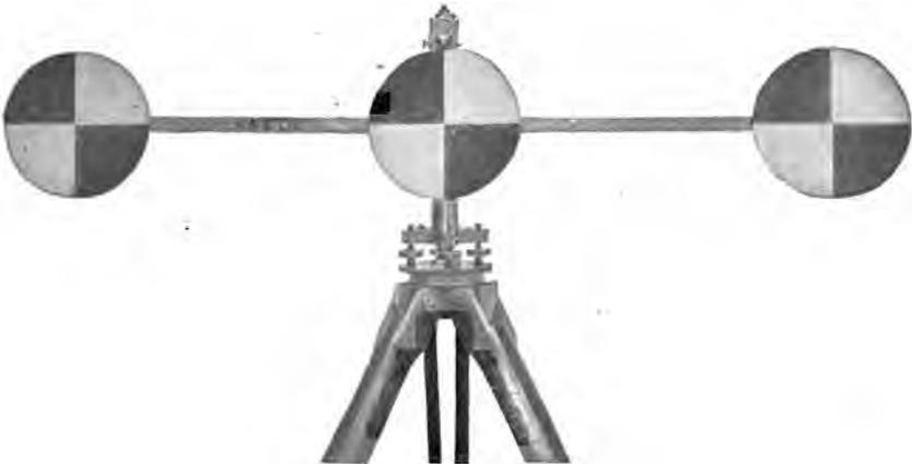
NOTWITHSTANDING that the idea of employing a horizontal bar with or without discs or targets placed in front of an observer provided with a transit, for ascertaining the distance between the target and the transit by means of the angle subtended by the bar or the discs, is probably, like the Italian Stadia, about a century old,—it yet seems to me that it has not received the attention which it deserves. This may be due to the sup-
