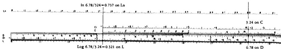
First, divide 6.78 by 3.24 in the usual way using C and D scales. Move cursor over 1 of C. Read  $\ln 6.78/3.24$  on Ln and read  $\log 6.78/3.24$  on L. If L scales are on the slide, close ruler (move slide so C and D indexes coincide) before reading from Ln or L. Or, if you prefer, first set slide so 1 of C is over 3.24 on D. Move hairline over 6.78 on D. Read logarithm from Ln or L.
