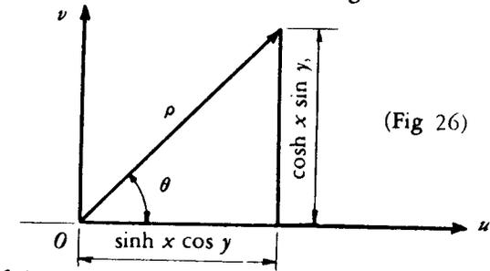
Methods of changing to the polar form  $\rho/\theta$  by use of the slide rule will now be explained. First, it should be noted that the real number  $y$  may be expressed in either radians or angular degrees. Since the graduations on the S and T scales are in terms of degrees, this measure is more convenient. A value of  $y$  given in radian measure should therefore first be converted to angular degrees.
