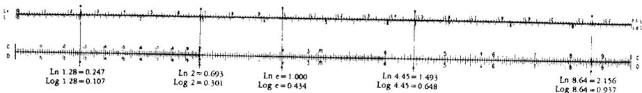
**Rule:** To find mantissas of logarithms: Set the number on the C (or D) scale, and read the mantissa for base 10 from L, or for base e from Ln. If L scales are on slide, set on C. If L scales are on body, set on D. Characteristic for base 10 is found by usual method. "Characteristic" for base e is explained in Section (e). Also, see below.
