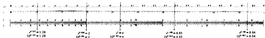
**Rule:** To find powers of  $e$  and of 10. Set the exponent of  $e$  on Ln, or of 10 on L, and read the power on C (or D). If L scales are on slide, use C; if they are on body, use D. The decimal point of the answer is found by special rules. See Section (f). Also see below.
