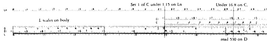
(i) **Division with powers.** Remember that division is the opposite of multiplication. The scales pictured in Section (h), on page 11, are set to divide 530 by  $e^{1.15}$ ; that is, to find  $530/e^{1.15}$  using D and C, or  $530 e^{-1.15}$ , using D and CI.
