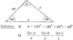
Set 48° on the S scale to 30′ on the D and then against 64° and 68° on Scale S you will be able to read off 36,3′ and 37.4′ on scale D.
