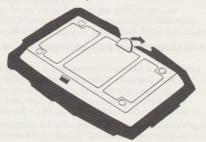
The exposed metal contacts on the battery pack are the battery terminals. Care should always be taken to prevent any metal object from coming into contact with the terminals and shorting the batteries.
