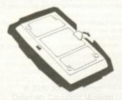
The metal contacts on the battery pack (where charger and calculator plug in) are the battery terminals. Care should always be taken to prevent any metal object from coming into contact with these terminals and shorting the batteries.
