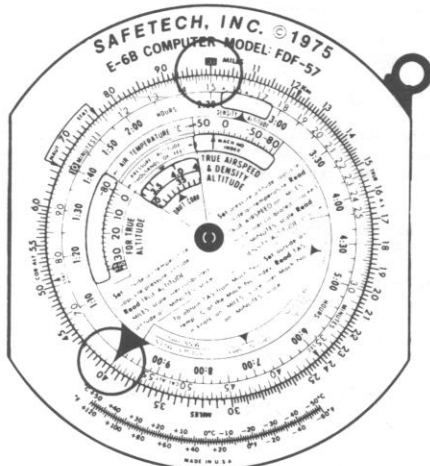
Figure 16. Off-Course Correction to Parallel
