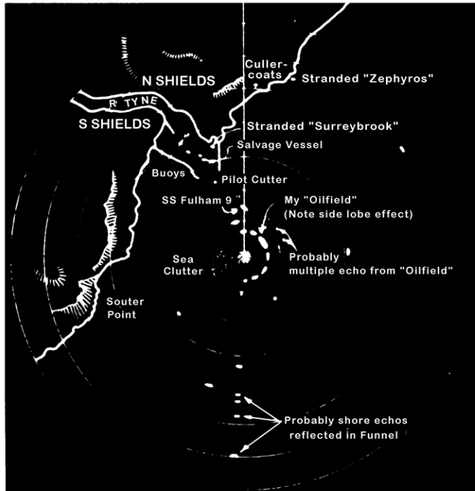
Figure 4.10 - Normal, indirect, multiple, and side echoes.
