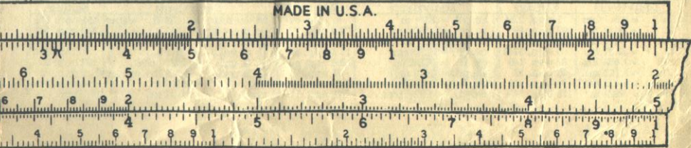
left index of C scale set over 2 on D scale.
