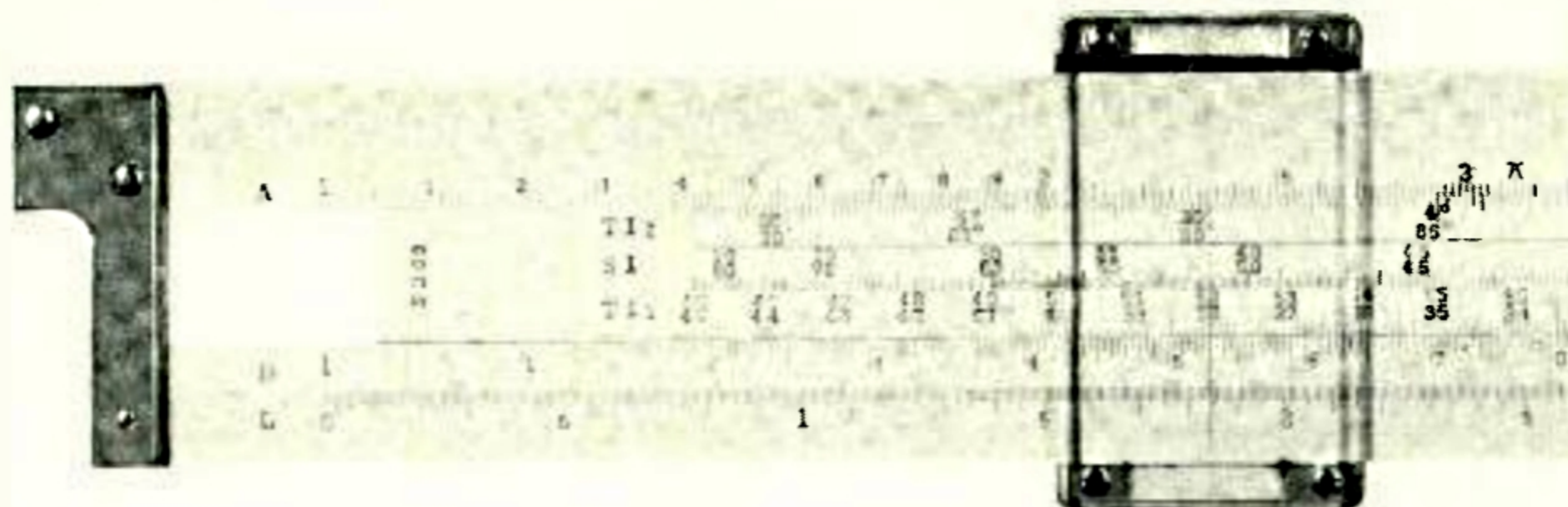
Fig. 3—Beginning of a conversion from rectangular to polar coordinates. When the slide is set on 1195 and the hair line on 1530 on scale D, angle \theta is given as 52^\circ on scale TI_1 . The later example is also illustrated here. With the slide set on 119.5 and the hair line on 1530, the angle is read on scale TI_2 — 85^\circ 32'
