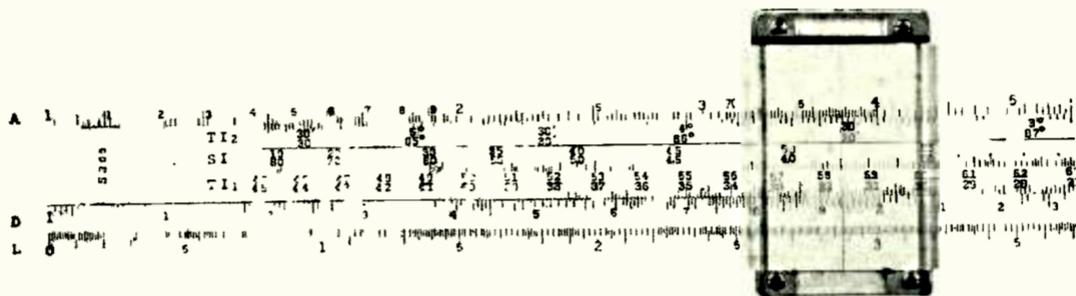
Fig. 4—With \theta learned, the slide is left at 1195 and the hair line moved to 52^\circ on scale SI. Then the vector r is given on scale D; its value is 1942
